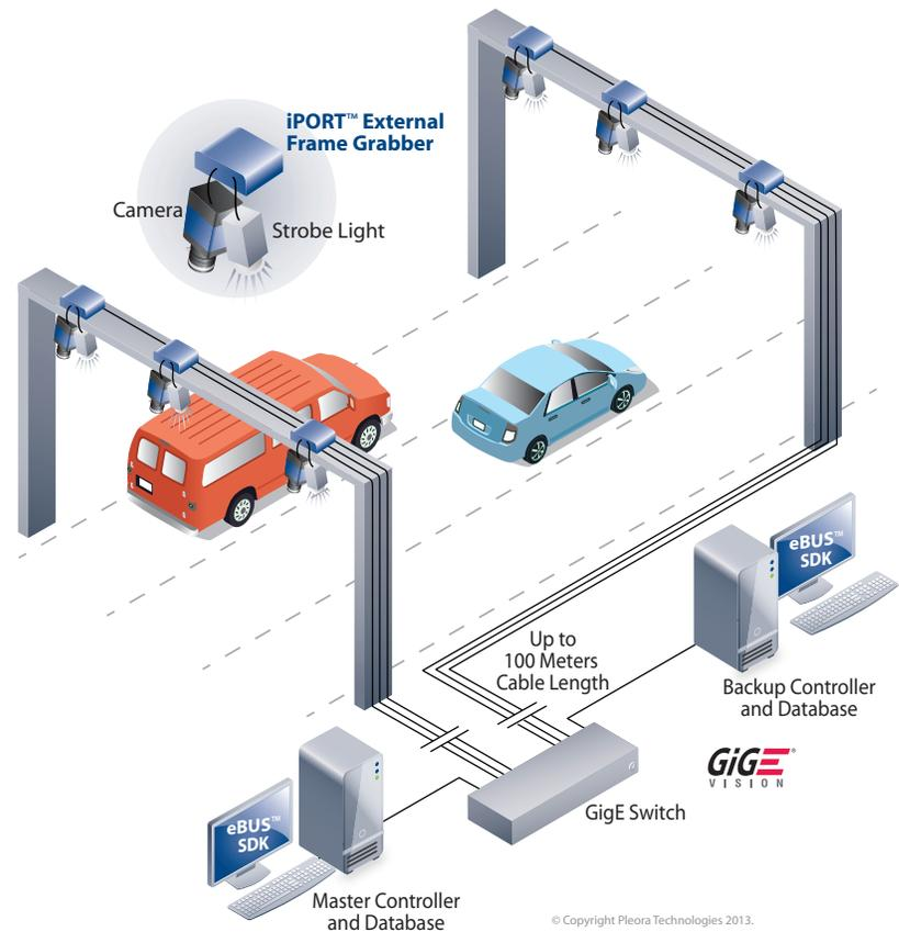
Diagram 1: In a free flow tolling system, external frame grabbers convert image feeds from existing Camera Link or analog cameras into a GigE Vision-compliant video stream.
